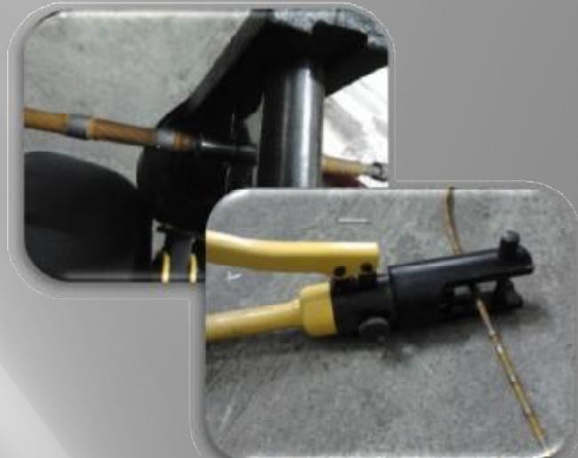
**Cut the wire with cutting wheel before jointing to obtain clean fractures, do not use scissors.**
