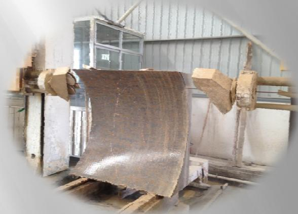
The wire and guiding wheels must be mounted symmetrically, in parallel and steadily.
