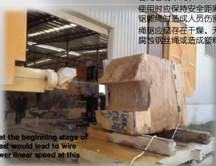
**Limit the down feed at the beginning stage of cutting, cutting too fast would lead to wire jamming, also use lower linear speed at this stage.**
