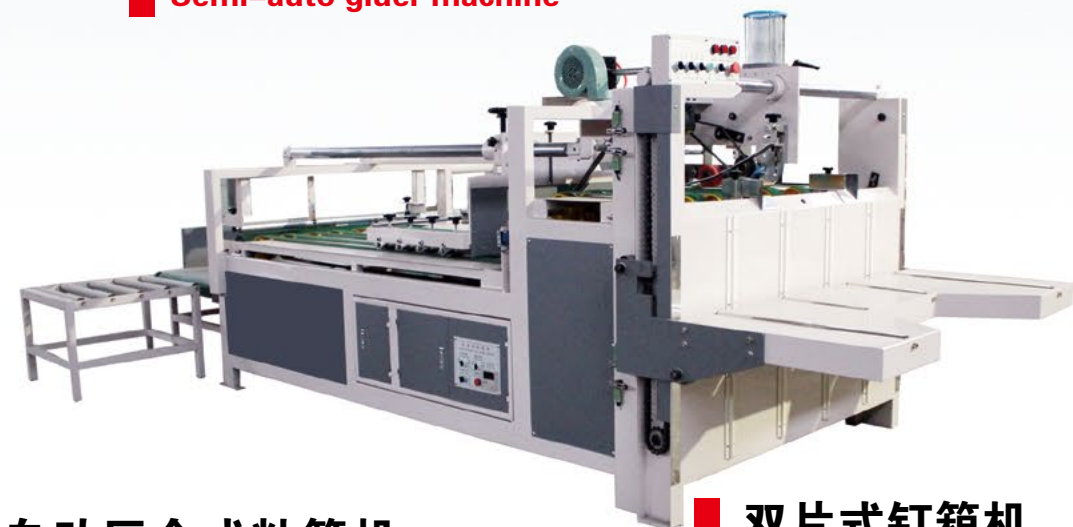
半自动压合式粘箱机 Semi-auto pressure folder gluer machine
