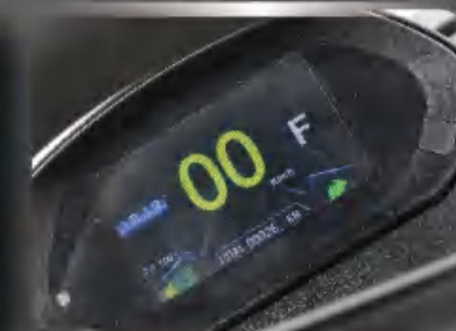
Instrument Cluster, with Speedo, Turn Lights, Battery Status and Backup Camera
