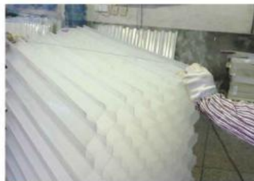
2. Use the Heating wire to cut the finished product along the diagonal
