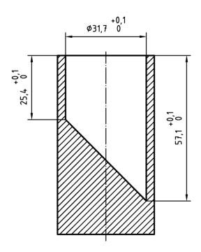
Figure 4 — Small parts cylinder
