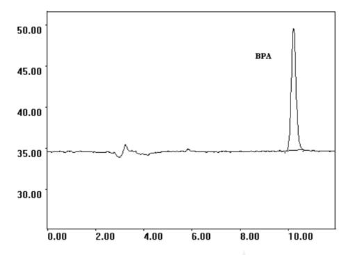
Figure B.1 – Chromatogram of BPA (absorbance (volt) v. retention time (min))
