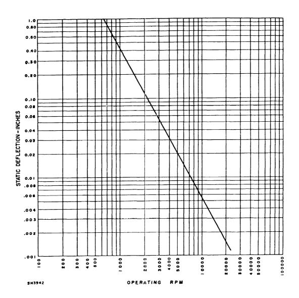
Figure 3 - Minimum static deflection of mounting for type II vibration test.
