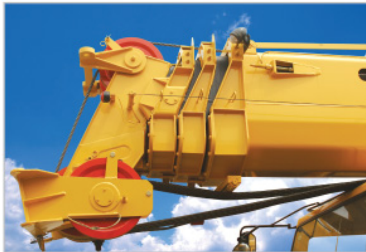
4 节八边形伸缩吊臂 4-section octagonal telescopic boom
