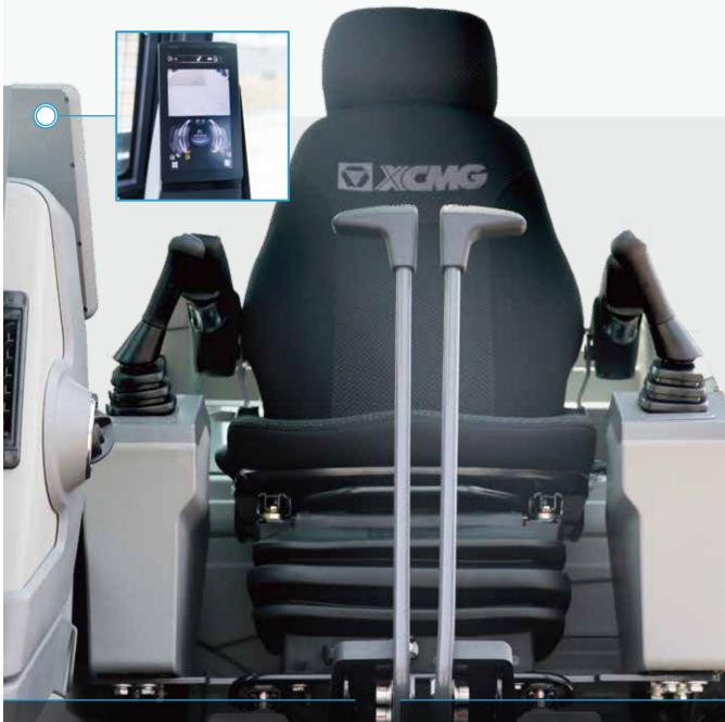
Imported silicone oil shock absorber can effectively isolate vibration and reduce driver fatigue.
