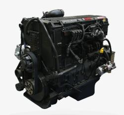
By adopting the engine which complies with national stage III emission standard and features with direct injection, four strokes, water cooling, turbocharging, air to air intercooler and six-cylinder, it can meet mining application requirements. Blending with proven, sturdy and durable parts and delicate manufacturing process, higher reliability and efficiency can be achieved.
