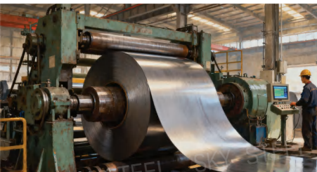
Uncoiling of steel coils
