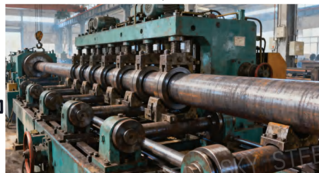
Steel pipe straightening
