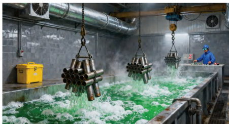
Pickling for rust removal
