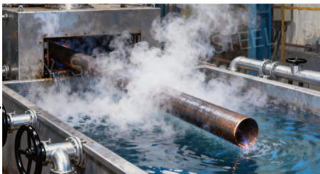
Cooling of welded pipes
