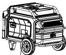
Oil service door
