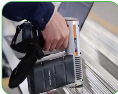
Coating Thickness Detection of Copper Busbars
