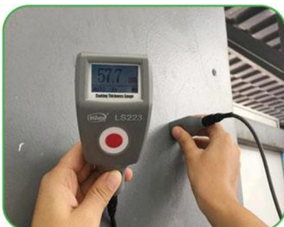
Paint Film Thickness Detection
