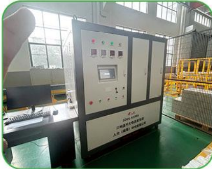
High-current temperature rise performance detector
