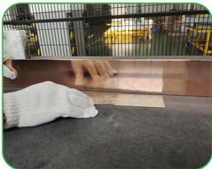
Flatness and Appearance Inspection of Copper Busbars
