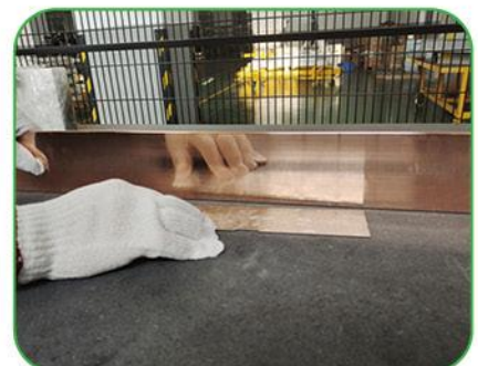
Flatness and Appearance Inspection of Copper Busbars
