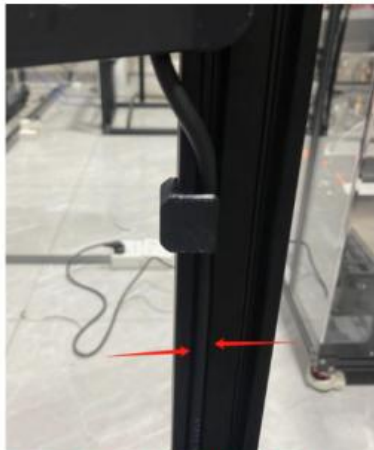
Insert the AC line (thick line) into the profile groove
