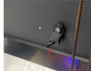
The resistor blackhead emerges 1cm from the fixing part
