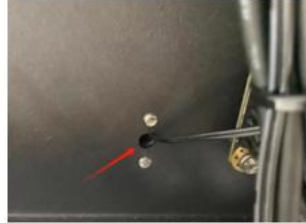
The thermistor black head is inserted from this hole, which is on the left side of the motherboard
