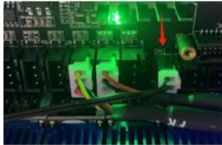
The terminal is inserted into the corresponding interface of THO
