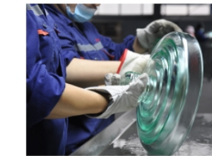
质检 Appearance quality inspection
