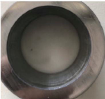
Spalling fatigue on raceway
