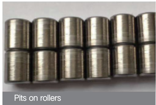
Spalling fatigue on rollers
