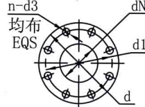
逆流进气口法兰尺寸 Cold Reflux Inlet Flange Size
