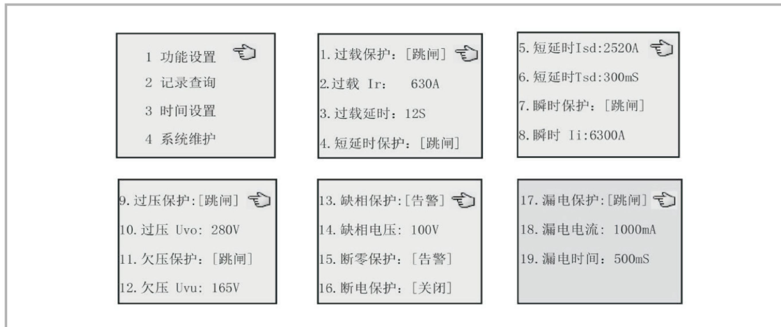
Figure 5: Operation Indication Interface
