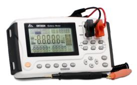
The CHT3554 battery tester is designed for large current and strong anti-interference to provide fast, complete and accurate diagnosis in internal resistance and voltage for backup UPS batteries and lead-acid batteries. Without stopping the instrument, CHT3554 can carry out online measurement and rapid diagnosis of deterioration of the batteries, greatly increasing the test efficiency. The built-in automatic data storage function can store up to 2400 sets of data.
