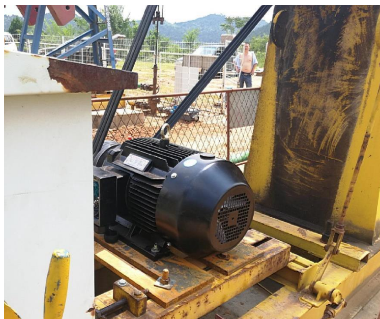
TYP160L-8-7.5kW permanent magnet synchronous motor
