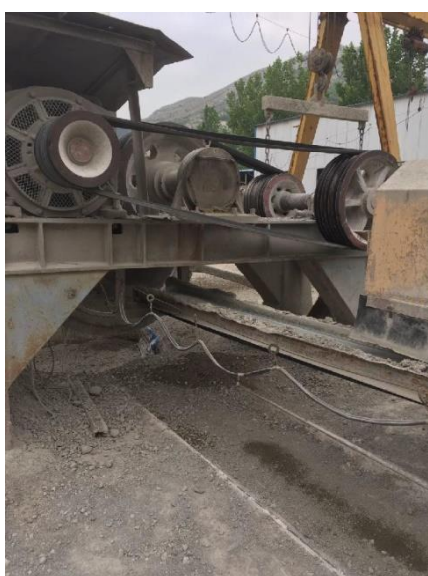
TYP280M-6-90kW Replacement YCT355-4E-132kW Motor
