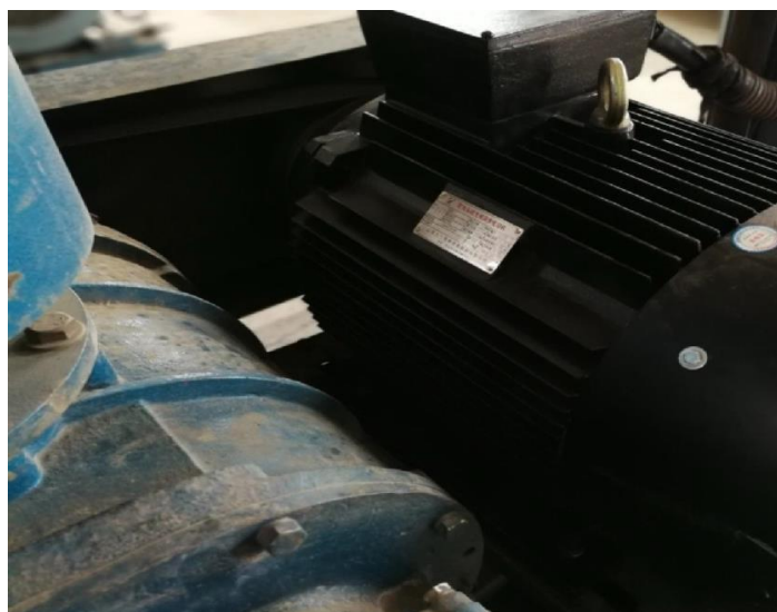
TYP280M-90KW Permanent Magnet Synchronous Motor
