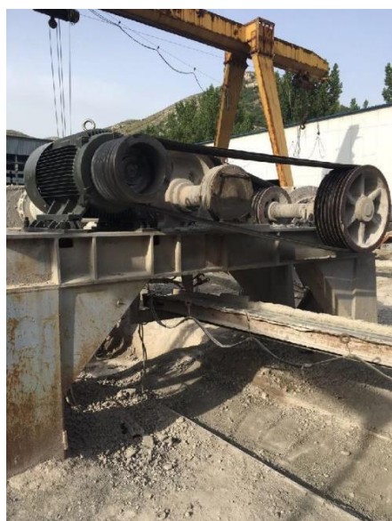
TYP280M-6-90kW Replacement YCT355-4E-132kW Motor
