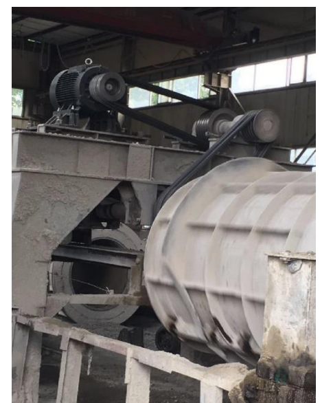
TYP225S2-6-45kW Replacement YCT355-4B-75kW Motor
