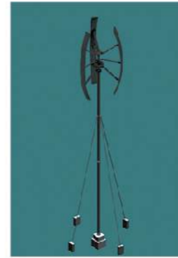
Guy Wire Tower
