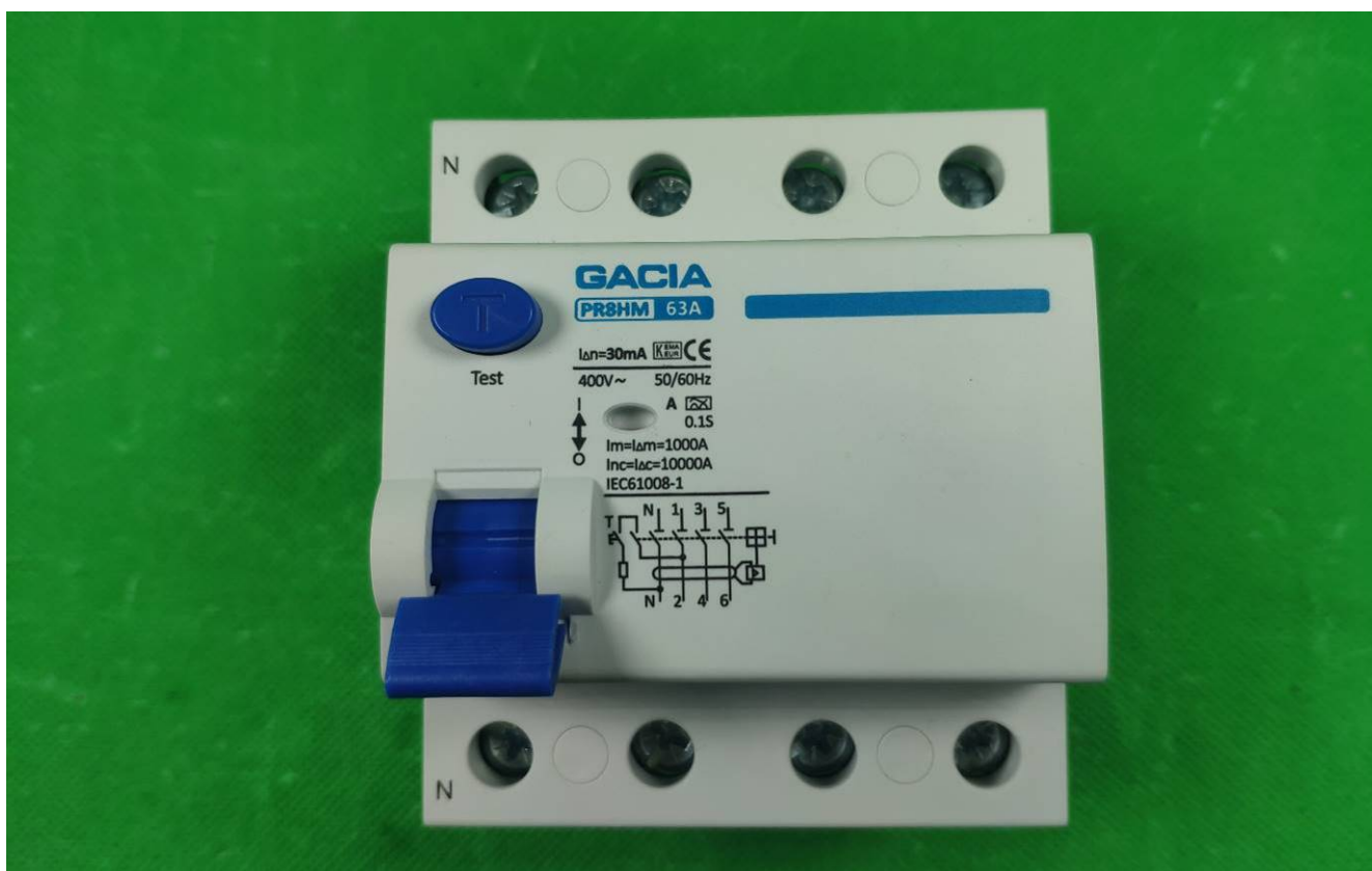
Front view, PR8HM / 3P+N / 63 A / 30 mA / A type
