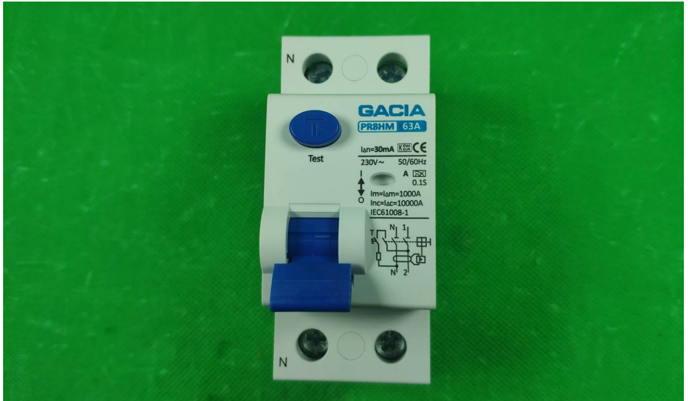
Front view, PR8HM / 1P+N / 63 A / 30 mA / A type
