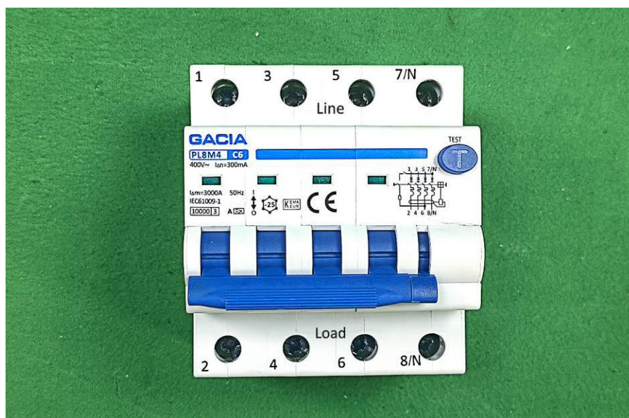
PL8M4, Front view, 4P / C6 / 300 mA / type A
