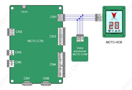
Figure 2-28 RS485 connection between the CTB, car display board, and voice announcer
