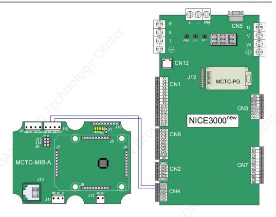
Figure 2-27 Connection between the NICE3000<sup>new</sup> and the MIB
