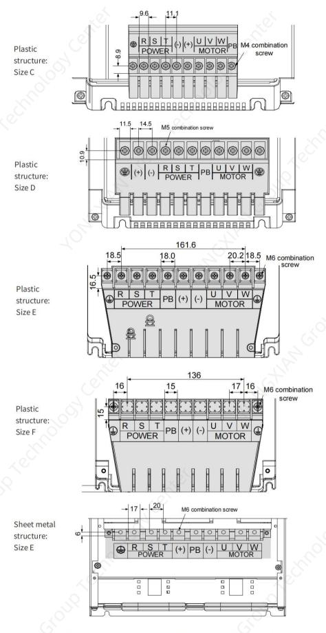
Figure 2-15 Terminal arrangement and size diagrams of Size C/D/E
