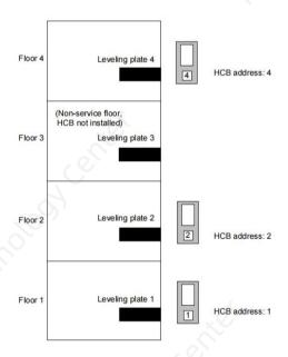
Figure 5-14 HCB installation and address setting
