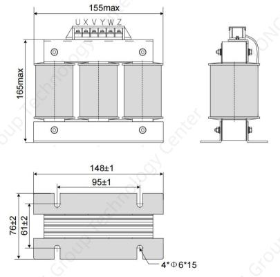
Figure 3-14 Physical dimension diagram of 20A AC output reactor
