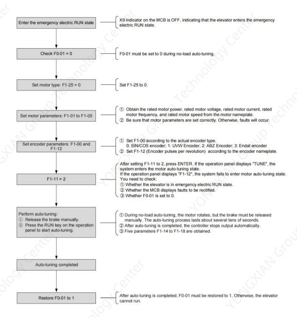
Figure 5-11 Asynchronous motor no-load auto-tuning
