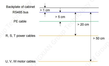
Figure 2-32 RS485 cabling diagram
