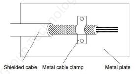
Figure A-5 Fastening the shield with the metal cable clamp
