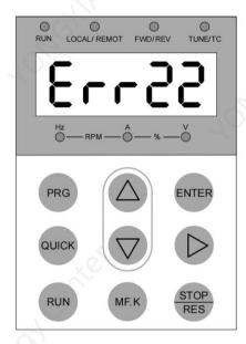
Figure 7-2 Fault code display on the operation panel
