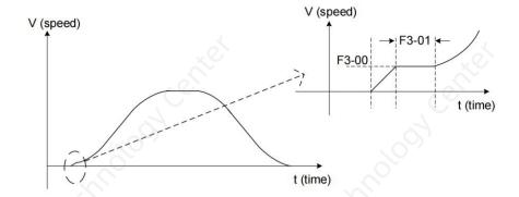
Bad riding comfort due to static friction may often exist in villa elevators. When there is large friction between the guide shoes and the guide rails, large static friction generates at the moment of startup, leading to bad riding comfort. Make the system starts up at the specified speed by setting these parameters to eliminate friction and improve riding comfort.
