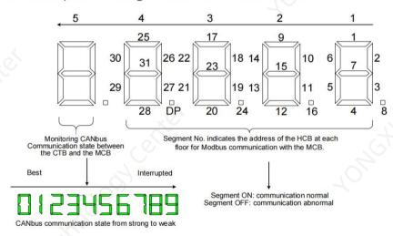
Figure 6-5 F5-32 communication state monitoring
