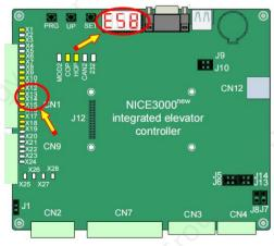
Figure 5-4 MCB state at faults during commissioning
