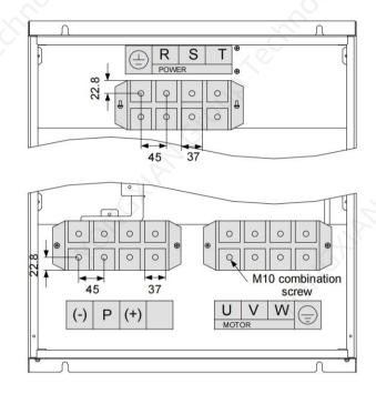
Figure 2-18 Main circuit cable terminal and size diagram of sheet metal structure, Size H
