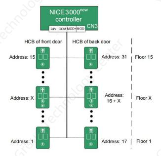
Figure 9-27 HCB setting of 15-floor opposite door control
