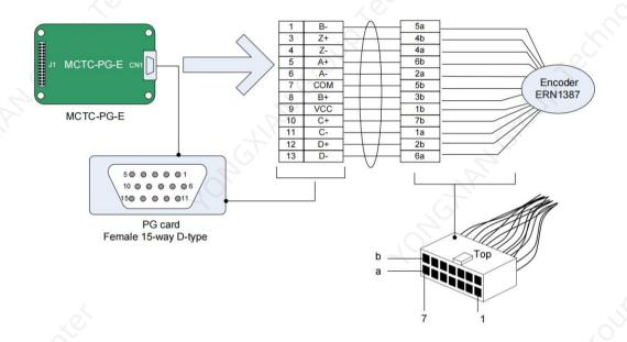
Figure 3-29 Connection between MCTC-PG-E and encoder ERN1387
