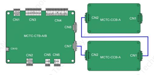
Figure 9-9 Wiring diagram 2 of disability operation box
