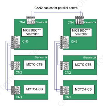
Figure 9-20 Wiring diagram of parallel control (via CN4)
