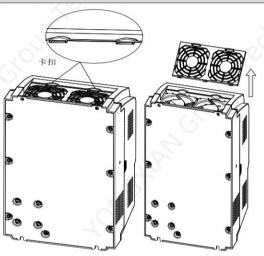
2) Lift the fan a little, disconnect the fan power cables from the socket, and then remove the fan.
