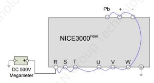
Figure 8-3 Main circuit insulation test
