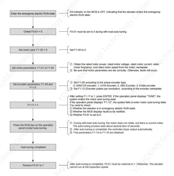
Figure 5-10 Asynchronous motor with-load auto-tuning
