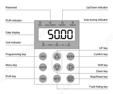
Figure 4-3 Diagram of the LED operation panel
