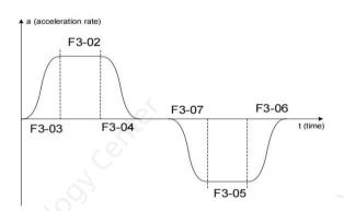
Figure 6-3 Acceleration rate curve
