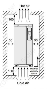
Figure 3-10 Mounting distance diagram of braking unit (unit: mm)
