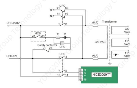
Figure 9-16 220 V UPS circuit
