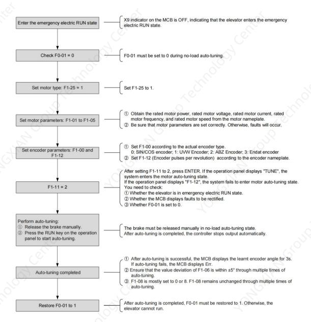
Figure 5-9 Synchronous motor no-load auto-tuning
