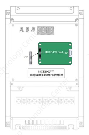
Figure 3-28 Appearance of the MCTC-PG card and its installation on the controller
