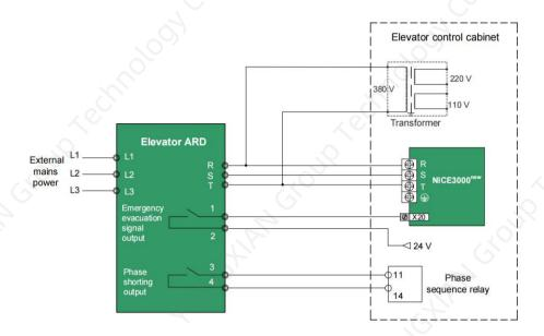
Figure 9-18 Wiring of three-phase (380 V) elevator ARD
