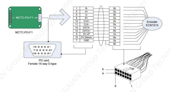
Figure 3-30 Connection between the PG card and encoder ERN1313
