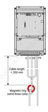
Figure 3-18 Installation of the common-mode filter
