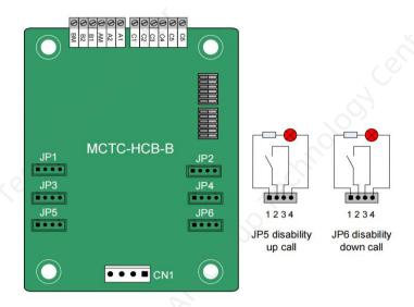
Figure 9-10 Wiring diagram of disability function enabled by HCB-B
