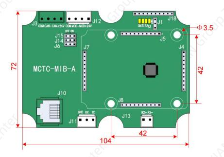
Figure 3-27 Appearance and dimensions of MCTC-MIB-A (unit: mm)
