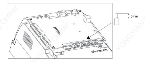
Figure 2-22 Control cable tubular terminal requirement
