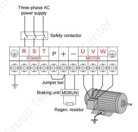
Figure 2-13 Main circuit connection diagram
