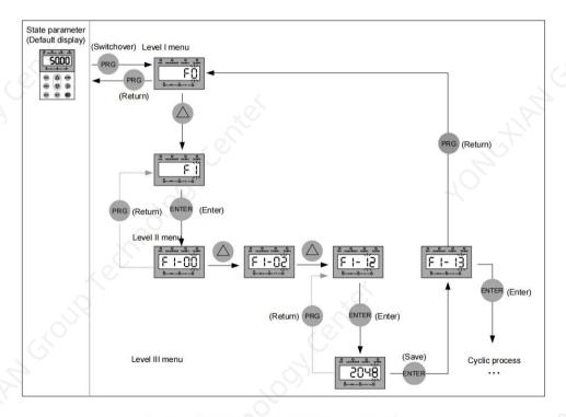
Figure 4-4 Parameter viewing procedure
