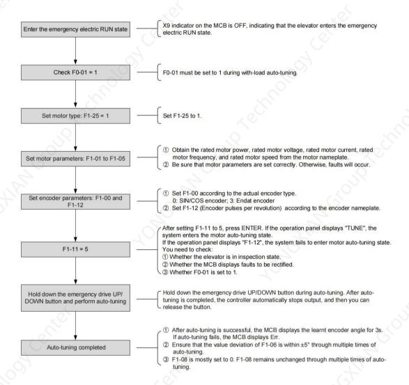
Figure 5-6 Synchronous motor static auto-tuning
