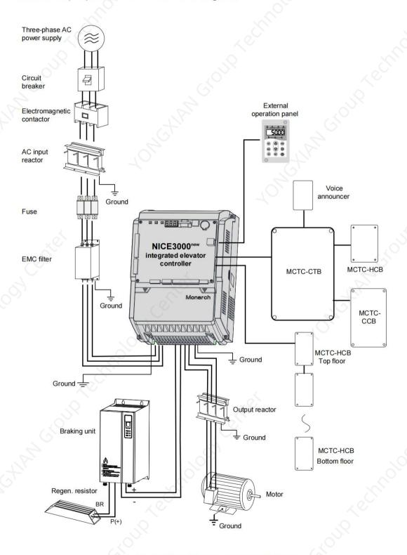
Figure 3-1 Peripheral device connection diagram
