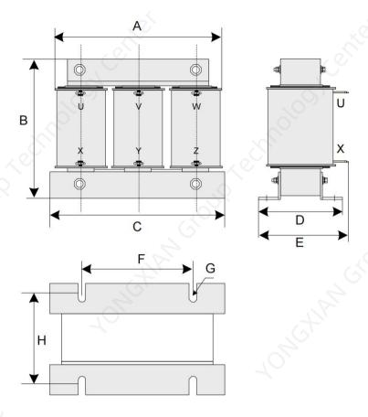
Figure 3-15 Physical dimension diagram of 50–120 A AC output reactor
