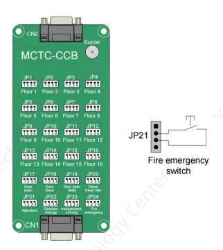
Figure 9-3 Wiring of firefighter operation signal input from CCB
