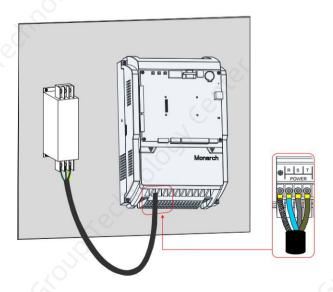
Figure 2-14 Installation on the conductive plane
