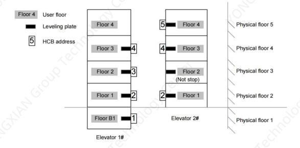
Figure 9-21 Floor diagram of two elevators in parallel control
