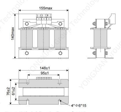
Figure 3-13 Physical dimension diagram of 15 A AC output reactor
