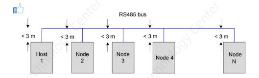
Figure 2-30 Branch connection structure
