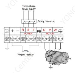
For models of 37 kW and above (F model 45 kW)
