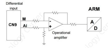
Figure 2-24 Analog differential input circuit
