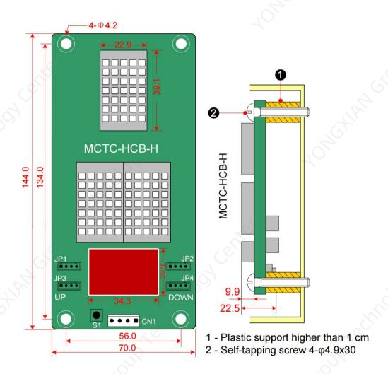
Figure 3-22 Appearance, dimensions, and installation method of MCTC-HCB-H
