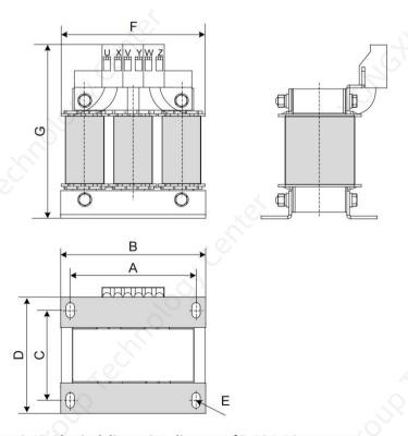
Figure 3-12 Physical dimension diagram of 5–10 A AC output react
