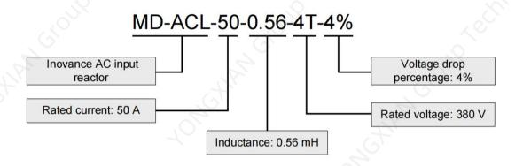
Figure 3-2 Designation rule of AC input reactor
