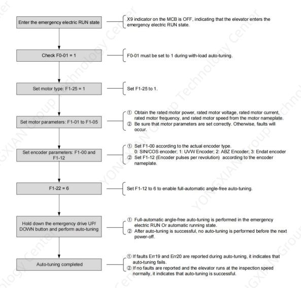
Figure 5-8 Full-automatic angle-free auto-tuning of synchronous motor
