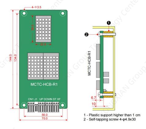
Figure 3-23 Appearance, dimensions, and installation method of MCTC-HCB-R1
