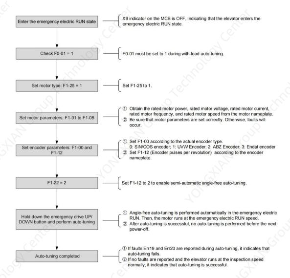
Figure 5-7 Semi-automatic angle-free auto-tuning of synchronous motor
