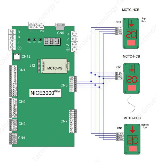
Figure 2-26 RS485 connection between the NICE3000<sup>new</sup> and the HCB
