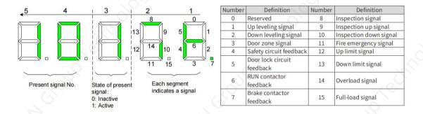
Figure 6-11 Example of FA-26 input state
