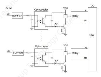
Figure 2-25 Relay output circuit
