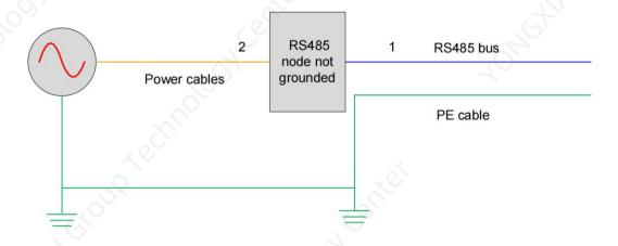
Figure 2-34 Suppressing external interference
