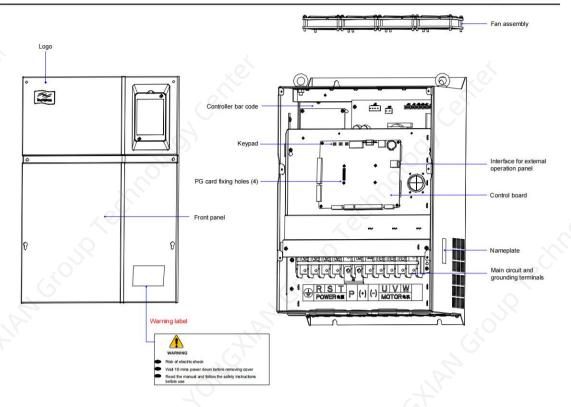
Figure 1-5 Component view of the sheet metal structure (NICE-L-C-4037 to NICE-L-C-4055)
