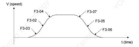
F3-02, F3-03, and F3-04 are used to set the running curve during which the elevator accelerates from startup to the maximum speed. If the acceleration process is too short causing bad riding comfort, decrease F3-02 and increase F3-03 and F3-04 to make the acceleration curve smoother. If the acceleration process is too long, increase the value of F3-02 and decrease the values of F3-03 and F3-04.
