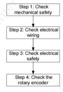
Figure 5-2 Flowchart of safety and circuit check before power-on
