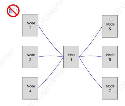
Figure 2-31 Star connection structure (wrong)
