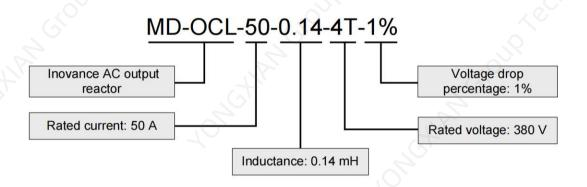
Figure 3-11 Designation rule of AC output reactor
