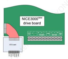
Figure 9-28 Connection between the controller drive board and the STO card The description of each STO terminal is as follows:
