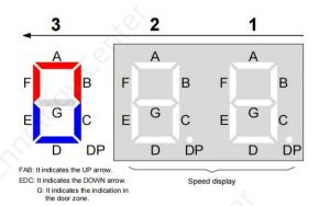
Note: When the speed is smaller than 1.000 m/s, the LEDs display ".xx m/s". When the speed is greater than 1 m/s, the LEDs display "x.x m/s". Therefore, the decimal places are different.
