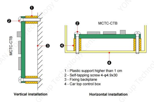
Figure 3-21 Mounting method of the CTB (unit: mm)
