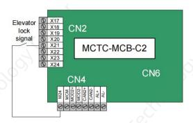
Figure 9-5 Wiring diagram of elevator lock signal input from MCB
