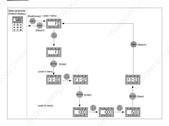
Figure 4-5 Parameter modification procedure
