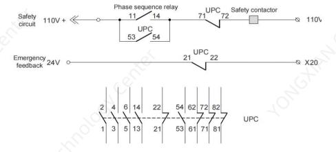
Figure 9-17 Various contacts of the contactors
