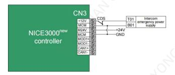
12 V input is added on the up and down leveling optoelectronic signal and power supply side. The 12 V power supply comes from the intercom emergency lighting. The action of the optoelectronic switch is driven by the emergency light upon power failure.
