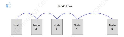
Figure 2-29 Hand-in-hand connection structure
