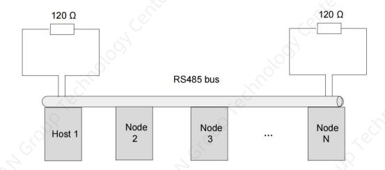
Figure 2-33 Correct termination resistor connection diagram
