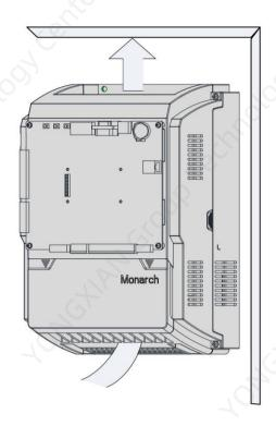
Figure 2-3 Heat dissipation diagram
