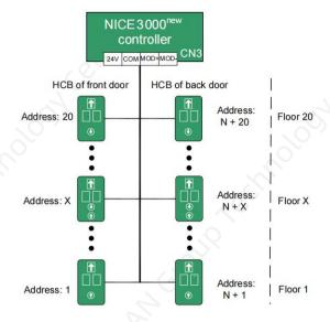
Figure 9-24 HCB setting diagram 1
