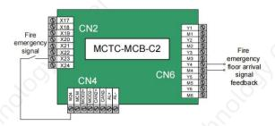
Figure 9-2 Wiring of fire emergency input signal from MCB
