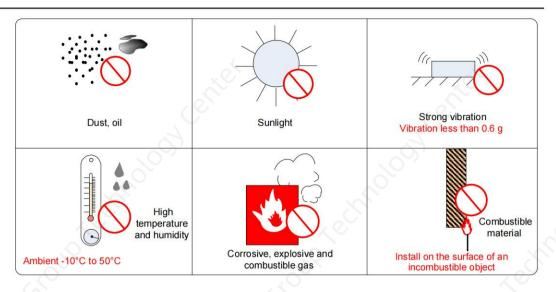
Figure 2-1 Schematic diagram of environment requirements
