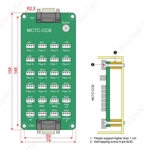
Figure 3-24 Appearance, structure and installation method of the CCB
