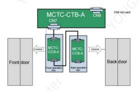
Figure 9-26 CCB wiring in mode 4
