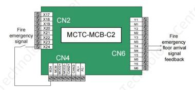
Figure 9-4 Wiring diagram of firefighter operation signal input from MCB
