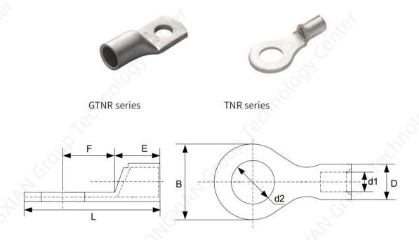
Figure 2-19 Dimensions of TNR series cable lugs
