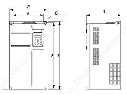
Figure 2-9  $\,$  [F model] Overview and installation dimensions of the sheet metal structure  $\,$  45–75 kW
