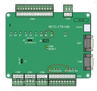
Figure 5-12 Input/output state indicated by CTB signal indicators
