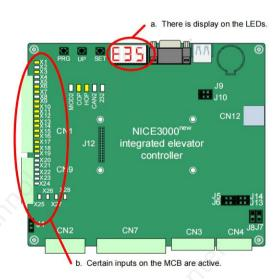
Figure 5-3 MCB display after normal power-on
