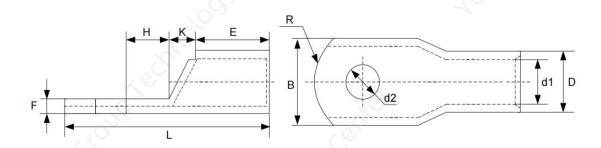
Figure 2-20 Dimensions of GTNR series cable lugs
