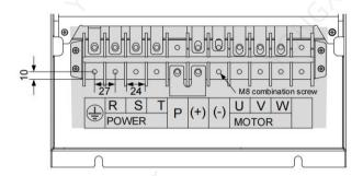
Figure 2-16 Main circuit cable terminal and size diagram of sheet metal structure, Size F
