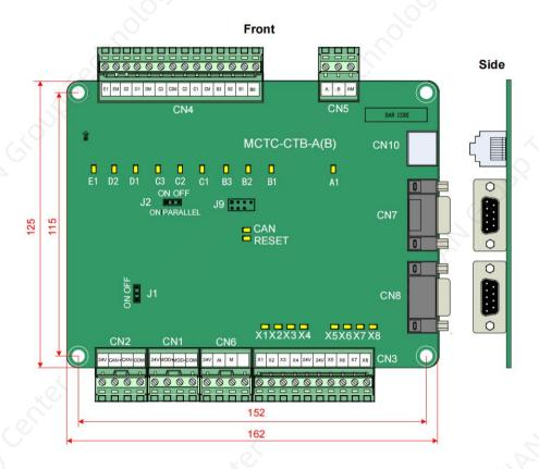
Figure 3-20 Appearance and dimensions of the CTB (unit: mm)
