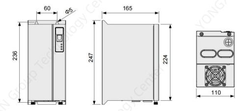
Figure 3-9 Appearance and mounting dimension diagram of braking unit (unit: mm)
