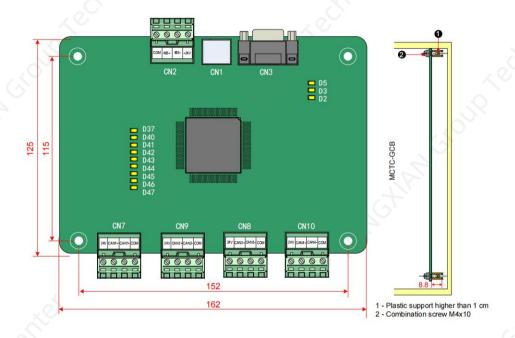
Figure 3-25 Appearance, dimensions, and installation method of the MCTC-GCB-A
