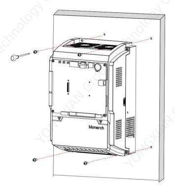
Figure 2-10 Wall-mounting diagram
