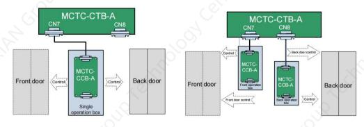
Figure 9-23 CCB wiring
