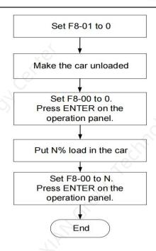
Figure 9-6 Analog load cell auto-tuning flowchart
