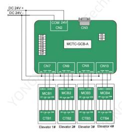
Figure 9-22 Wiring diagram of group control
