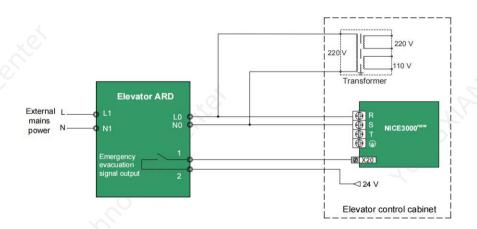
Figure 9-19 Wiring of single-phase (220 V) elevator ARD
