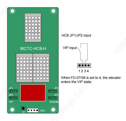
Figure 9-11 Wiring diagram of VIP enabled by HCB
