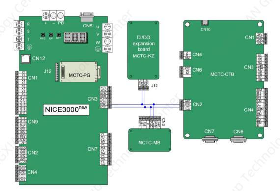
Figure 2-36 CAN connection between the NICE3000<sup>new</sup> and the CTB, DI/DO expansion board and equipment-roomless monitoring board
