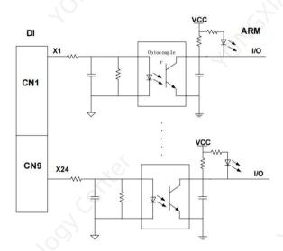
Figure 2-23 DI circuit
