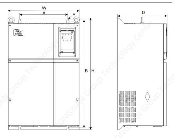
Figure 2-7 Overview and installation dimensions of the sheet metal structure 37–160 kW
