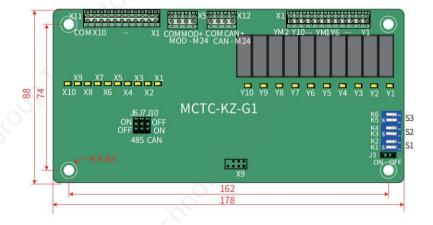
Figure 3-26 Appearance and dimensions of the MCTC-KZ-G1 (unit: mm)
