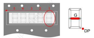
Figure 9-7 Monitoring of full-load/overload signals in F5-35
