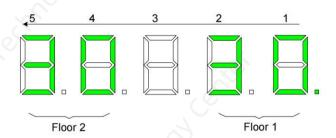
As shown in the preceding figure, the left two LEDs and the right two LEDs respectively show the adjustment bases of the first floor and second floor. If the value is larger than 30, it is upward leveling adjustment; if the value is smaller than 30, it is downward leveling adjustment. The default value "30" indicates that there is no leveling adjustment. The maximum adjustment range is  $\pm 30$  mm.
