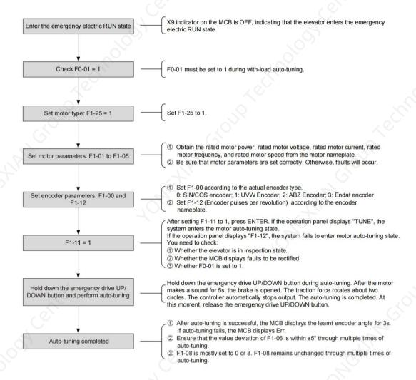
Figure 5-5 Synchronous motor with-load auto-tuning
