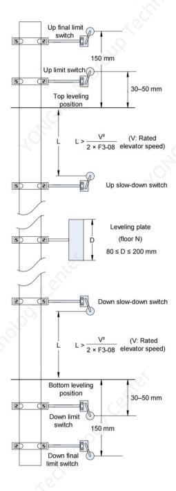
Figure 2-37 Arrangement of shaft position signals
