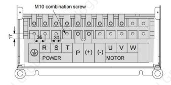
Figure 2-17 Main circuit cable terminal and size diagram of sheet metal structure, Size G
