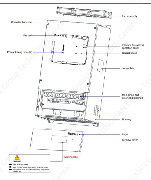
Figure 1-4 Component view of the sheet metal structure (NICE-L-C-4018 to NICE-L-C-4030)
