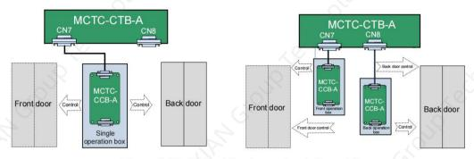
Figure 9-25 CCB wiring in modes 1, 2, and 3
