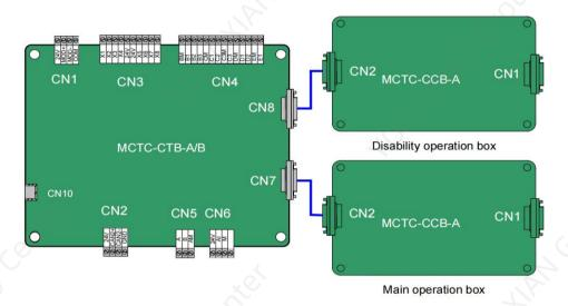
Figure 9-8 Wiring diagram 1 of disability operation box
