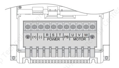
Figure 2-12 Main circuit terminal arrangement
