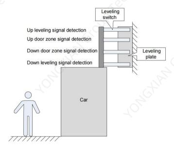
Figure 2-38 Installation of leveling signals
