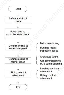
Figure 5-1 Overall commissioning flowchart of the NICE3000<sup>new</sup>
