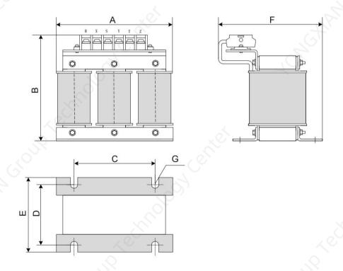
Figure 3-3 Physical dimension diagram of 7-10 A AC input reactor
