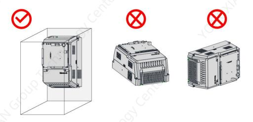
Figure 2-4 Mounting orientation of the controller
