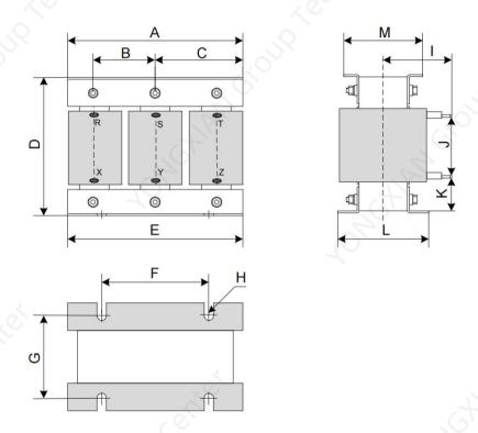
Figure 3-4 Physical dimension diagram of 15-50 A AC input reactor
