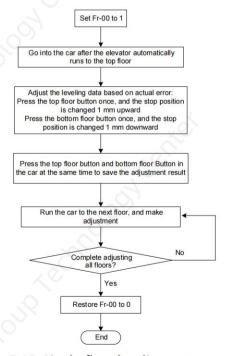
Figure 5-18 Single-floor leveling accuracy adjust
