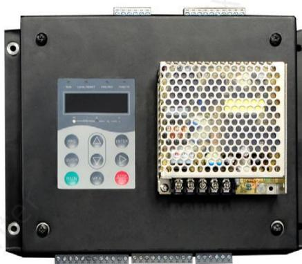
Figure 1-1 Physical appearance of the MCTC-PES-E1 (a control board fixed inside the black housing)
