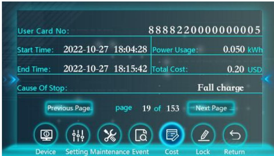
SINO APP query method: open SINO APP → Charging → Add new device → select SN → Connect → enter the maintenance password → Record, as shown in the figure below:
