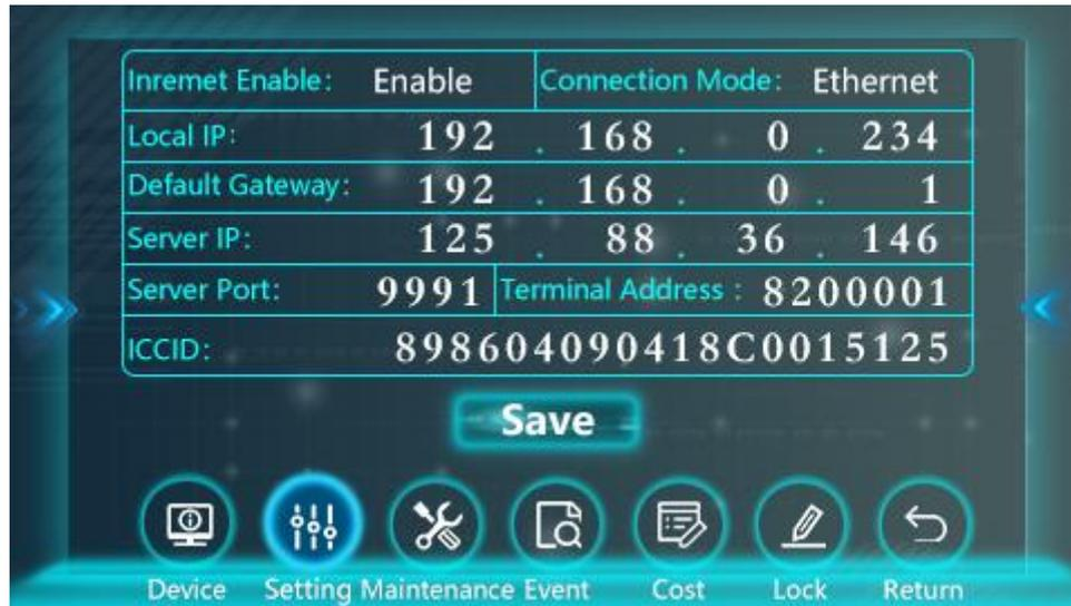
② SINO APP configuration: open SINO APP → Charging → Add new device → select SN → Connect → enter the maintenance password → Modification → Network parameters → Background enable: Enable → Connection method: Ethernet;
