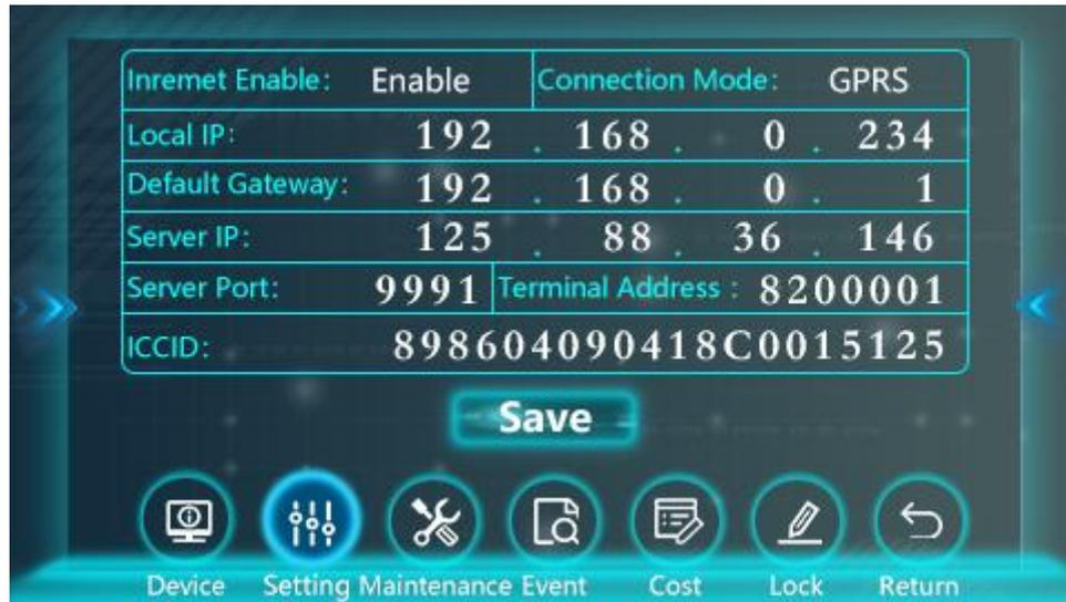
② SINO APP configuration: open SINO APP → Charging → Add new device → select SN → Connect → enter the maintenance password → Modification → Network parameters → Background enable: Enable → Connection method: GPRS;
