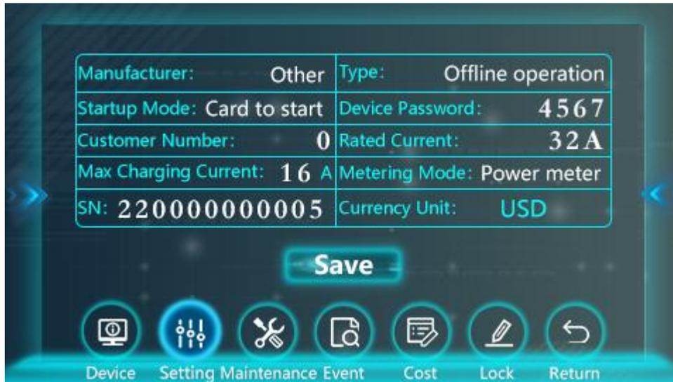
SINO APP restriction method: open SINO APP → Charging → Add new device → select SN → Connect → enter the maintenance password → Charging current → the limitable range is 6A~rated current, as shown in the figure below:
