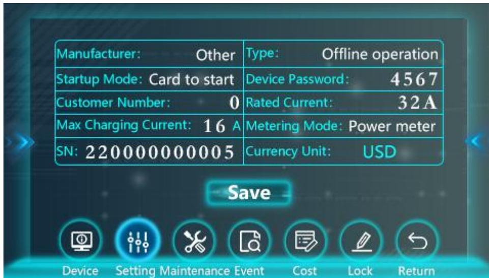
SINO APP modification method: open SINO APP → Charging → Add new device → select SN → Connect → enter the maintenance password → Modification → Device parameters → change Password; it can be modified to 1~8 digits, please keep the password after modification, as shown in the figure below Shown:
