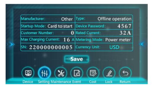
SINO APP modification method: open SINO APP  $\rightarrow$  Charging  $\rightarrow$  Add new device  $\rightarrow$  select SN  $\rightarrow$  Connect  $\rightarrow$  enter the maintenance password  $\rightarrow$  Modification  $\rightarrow$  Device parameters  $\rightarrow$  change Password; it can be modified to 1~8 digits, please keep the password after modification, as shown in the figure below Shown:
