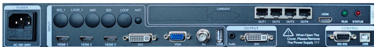
Figure 1 -- Video Controller Rear Panel
