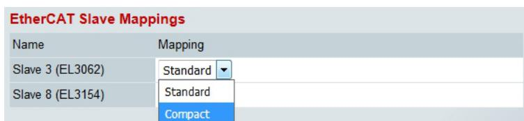
⇒ You have successfully set the mapping for the EL3062 EtherCAT Terminal. Restart the EK3100 Bus Coupler for the settings to take effect after reboot.
