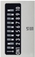
Fig. 15: DIP switch S001: left off "0", right on "1"
