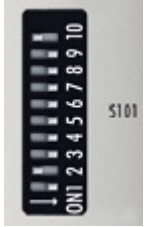
Fig. 14: DIP switch S001: Left off "0", right on "1"
