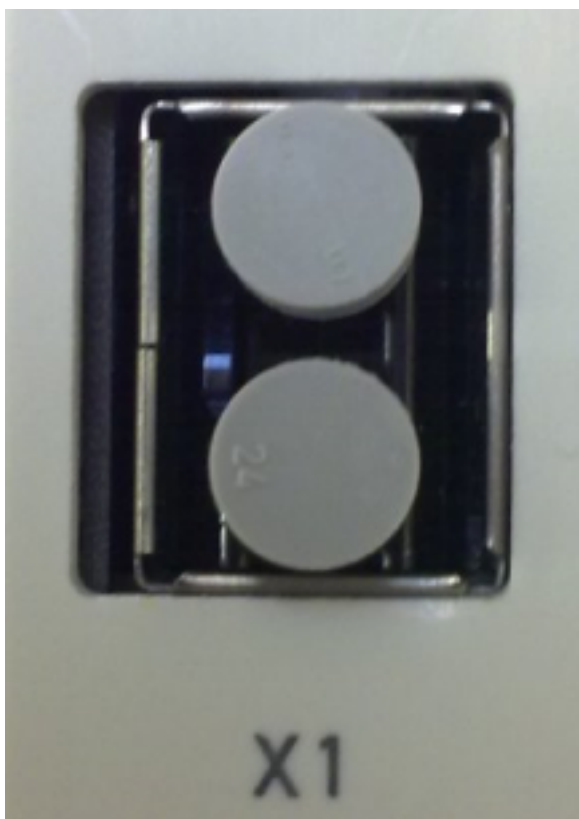
Figure: Blind plugs in unused sockets
