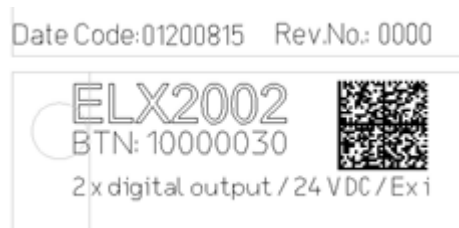
Fig. 138: ELX2002 with Beckhoff Traceability Number (BTN) 10000030 and Date Code 01200815
