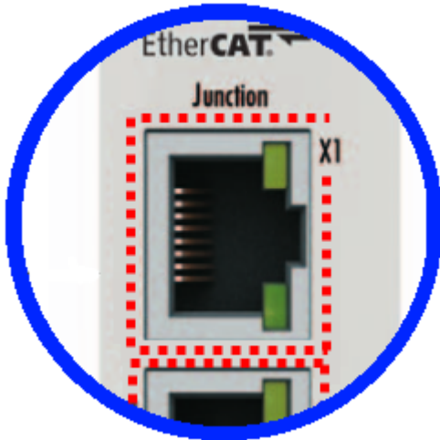
Fig. 36: Identification of FHC port at EK1122-0080 and EK1101-0080
