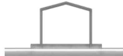
Gable roof style
