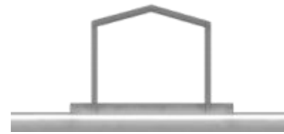
Gable roof style
