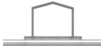
Gable roof style
