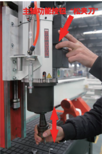
Spindle functional button “loosen and clamp tools” .
