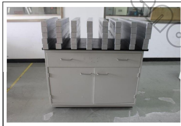
Cabinet Load Test
