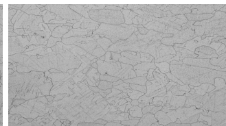
Microstructure in heat-treated state (left: XY direction; right: Z direction)
