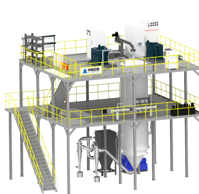
The powder metallurgy technology and equipment production line-- Non-Vacuum Gas Atomization (AVI-GA)
