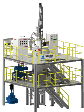
The powder metallurgy technology and equipment production line-- Electrode Induction Gas Atomization (AVI-EIGA)
