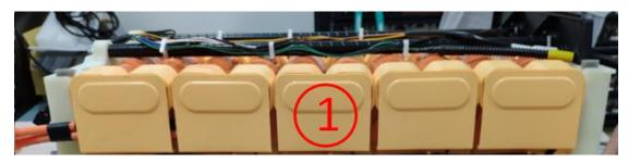
7.2 Install the main positive and negative insutating cover forinsulating protection.安装总正、总负绝缘帽,进行绝缘防护。
