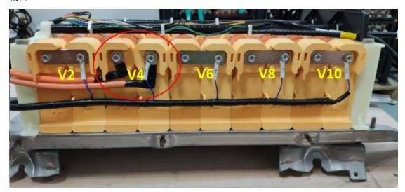
6.2 Install the positive connector wire and the voltage collection wire harness #V11 . Note: The main positive wire harness of sample is in the form of a wire harness, will be optimized to connector copper bar in the future. (安装正连接线及电压采集线束 V11。注:前期样品总正线束采用线束形式,后续优化为连接铜牌)。
