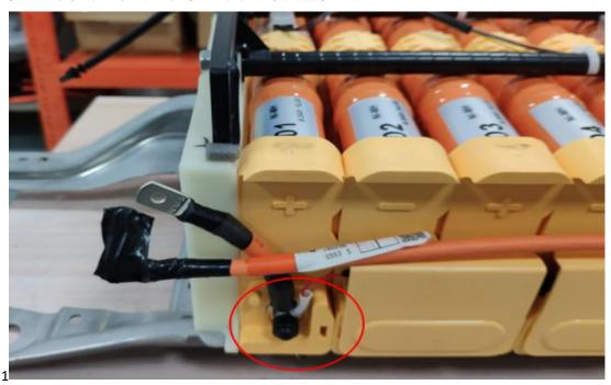
6.3 Install negative connector wire and the voltage collection wire harness #V01. Note: the main negative connection wiring harness adopts
