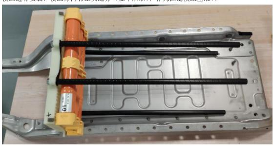
4.2 Install the temperature probe on the module: 01, 06 and 10 top buttons, and fixing the wire harness. Installation method of temperature
