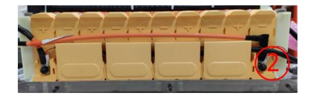
8. Install the plugs of voltage collection wire and temperature sensor according to the original position. (按原位置安装电压采集接线插头和温度传感器插头)。
