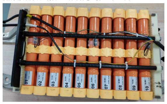
4.3Before the bottom screws of module are tightened, the plastic splints on both sides need to be loosened suitably to facilitate the adjustment o f the bottom screws hole. After the bottom screws are all screwed in, fix the plastic splints on both sides , and finally tighten the bottom bolts. 底 部螺丝紧固前,两侧塑料夹板适当松动,以方便调整底部螺丝孔位,底部螺丝全部拧入后,将两侧塑料夹板紧固,最后再拧紧底部螺栓
