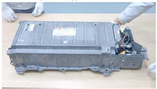
10. T Put the battery pack back to the vehicle, and connect the main wire of cathode pole and anode pole in correct position. (the correct position are marked with red circle in the follow picture). (完成组装的电池组件, 然后放回车辆,正确连接正负主线一标有红圈的位置)。
