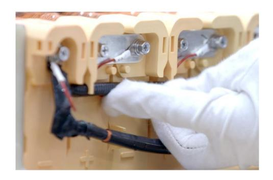
5.3 To Install the voltage collection wire into wire harness groove on the other side. (安装另一侧电压采集线束及连接铜牌)。
