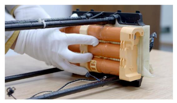
4.2 The temperature probe should be installed on the buckle of the bottom of the module #01, #07 and #14. (将温度探头安装在模组:01、07和14底部卡扣上)。
