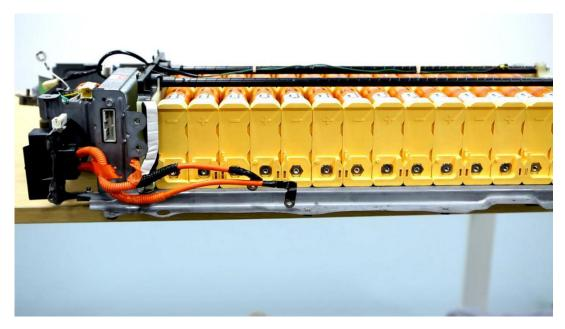
6.2 Install the original voltage collection wire #V15 of the anode pole connector wire. ( 安装原版正连接线电压采集线束 V15)
