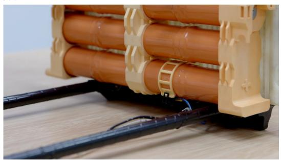
4.3 The temperature probe wires harness should be installed on the buckle of the bottom of the module #04 and #10. (将温度探头线束安装在模组 (04,10) 底部卡扣上)。
