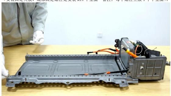
4.5 Tighten the screws at the bottom of module (Note: The torque of screw is  $5^{\circ}6N \cdot M$ ).将模组底部螺丝进行拧紧固定(注:铜牌螺丝扭力 $5^{\circ}6N \cdot m$ )。 Tighten the splint screws to fix the position. (将定位夹板螺丝进行拧紧固定)。 Tighten the splint screws at the bottom of module to fix the position.
