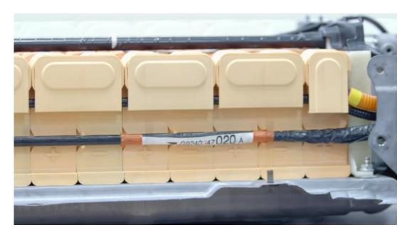
8. Install the plugs of voltage collection wire and temperature sensor according to the original position. (按原位置安装电压采集接线插头和温度传感器插头)。
