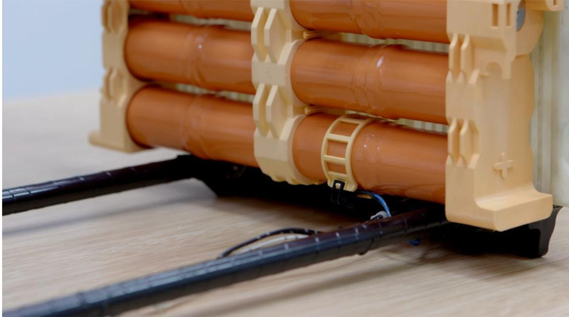
4.3 The temperature probe wiring harness should be installed on the buckle of the bottom of the module #04 and #10.
