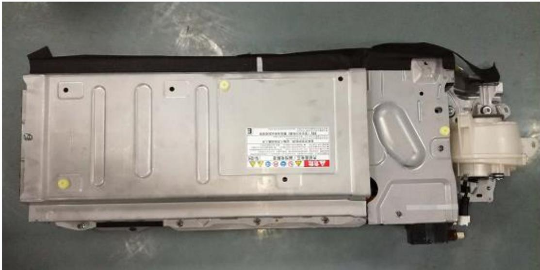
10. Put the battery pack back to the vehicle, and connect the main wire of cathode pole and anode pole in correct position. (the correct position are marked with red circle in the follow picture).
