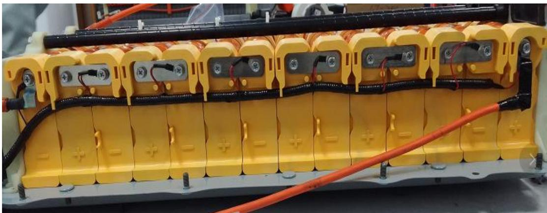
6. Install the wiring harness of cathode pole, the wiring harness of anode pole and safety wiring harness .
