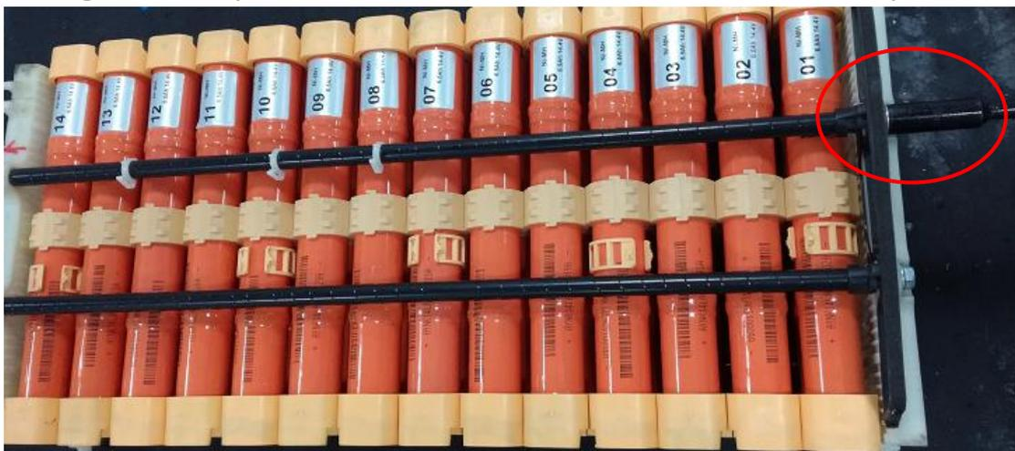
5. The installation of the connector copper bar and voltage collection wire.
