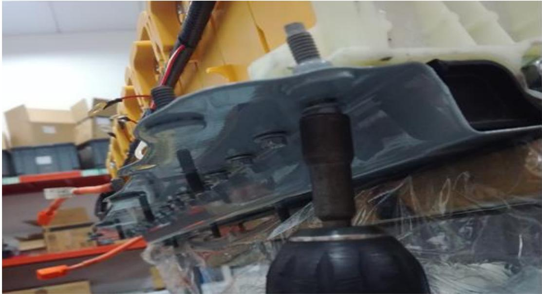
4.5 Tighten the splint screws at the bottom of module to fix the position.
