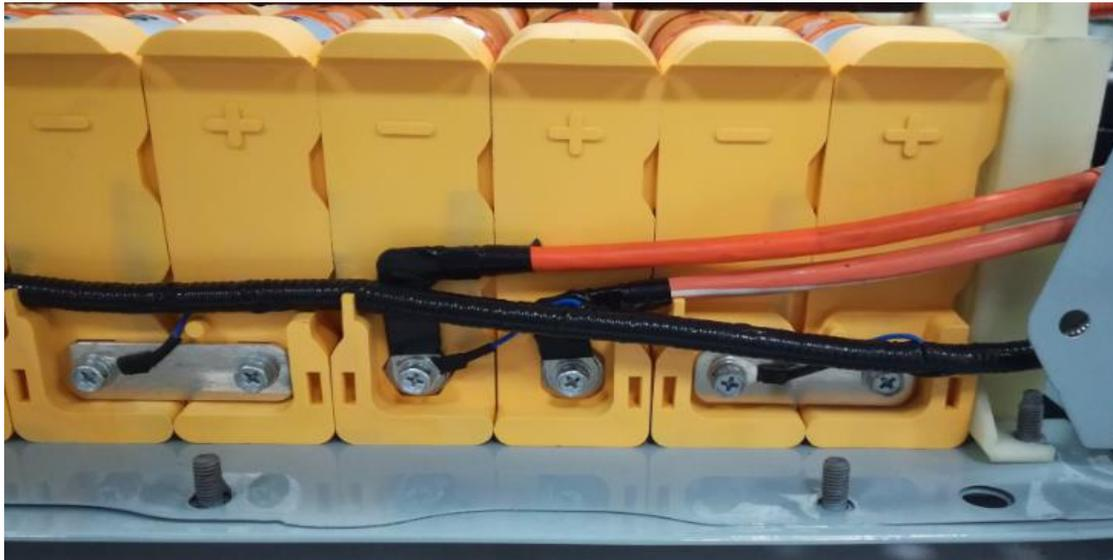
5.2 Immobilize the voltage collection wire into wiring harness groove.
