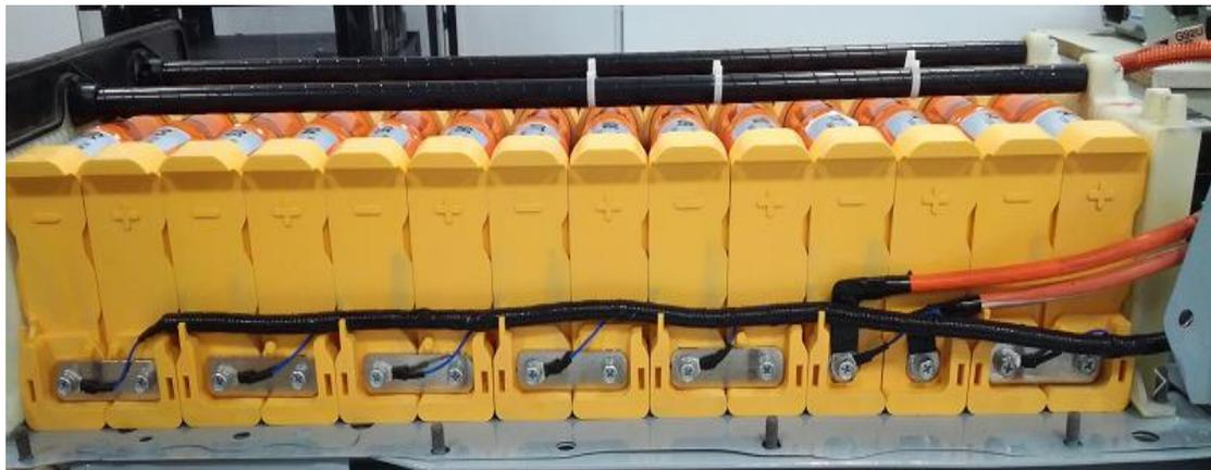
5.3 Install the voltage collection wire into wiring harness groove on the other side.
