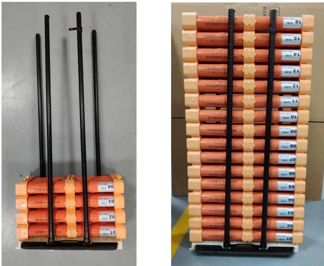
4.2 The temperature probe should be installed on the buckle of the bottom of the module #01, #08and #16.
