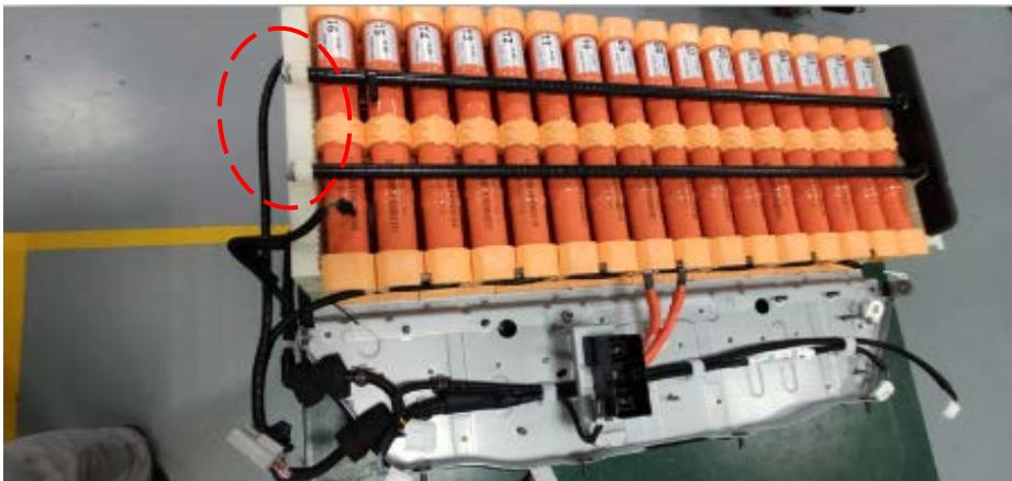
8. Install the original insurance connector on the position of voltage collection wire #V10 according to the red circle as showed in following picture. ( 安装原保险连接器，连接在08#、09#模组上，并将电压采集电路V8安装在08#模组上，如下图所示 )。
