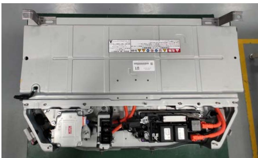
12. Check everything correctly after finishing all accessories installation , then install the original insurance component(MSD). ( 完整安装所有配件 , 正确检查一切后安装原保险(MSD) ) .
