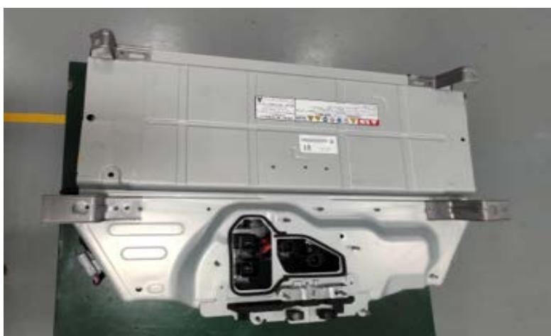
13. Put the battery pack back to the vehicle, and connect the main wire of positive pole and negative pole in correct position. ( 将完成组装的电池组件，然后放回车辆，正确连接正、负极主线 )。
