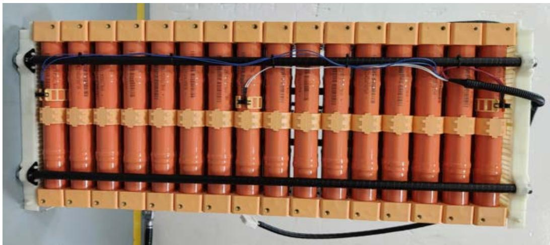
5. The installation of the connector copper bar and voltage collection wiring harness. ( 安装连接铜排及电压采集线束 )。
