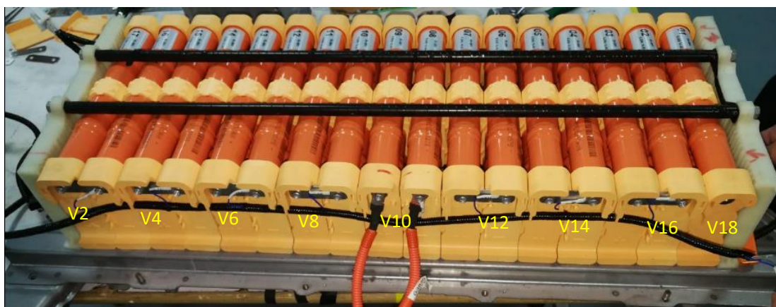
5.3 Install the voltage collection wire and connector copper car into wiring harness groove on the other side.
