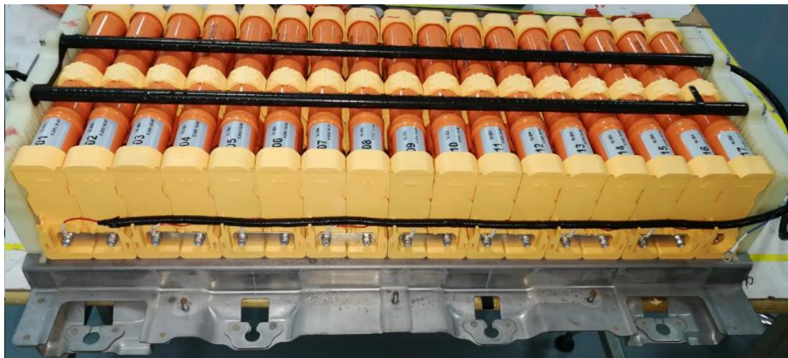
5.3 Install the voltage collection wire and connector copper car into wiring harness groove on the other side.
