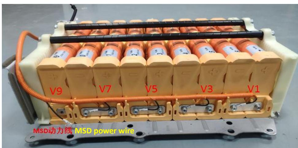
12. Install voltage collection wiring harness and copper busbar on the other side. Note: torque of bronze screw is 5 ~ 6N•m. (安装另一侧电压采集线
