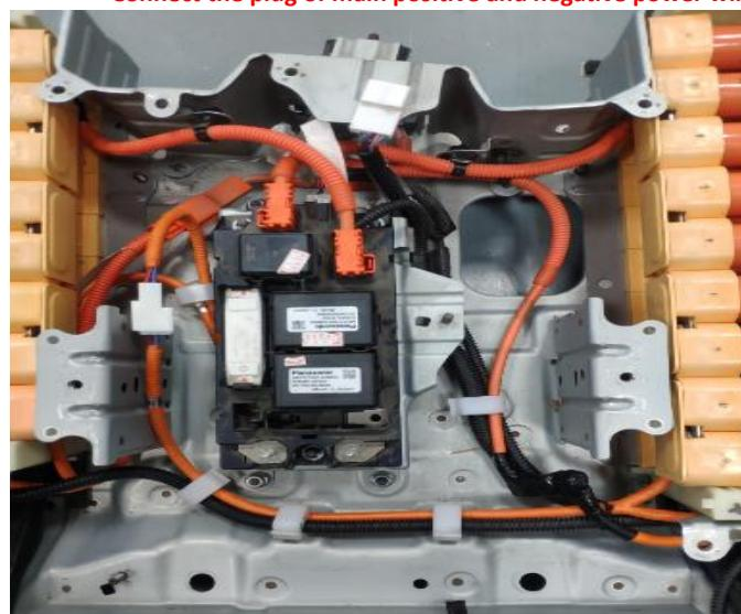
18. Install the cover plate of battery pack (安装电池组件盖板)。
