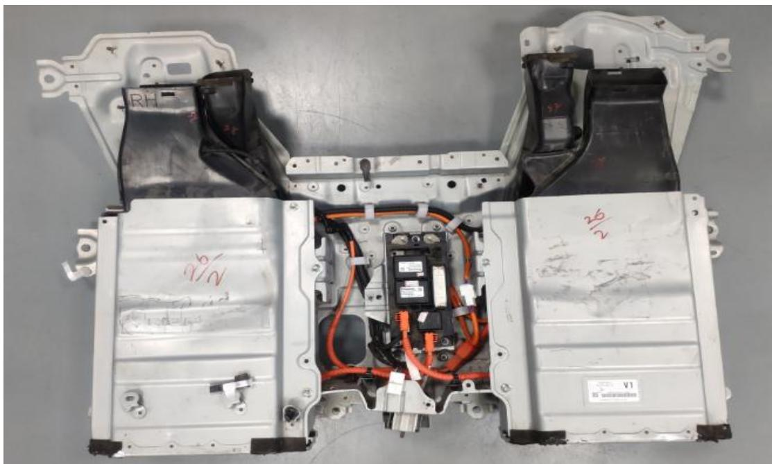
19. Put the battery pack back to the vehicle, and connect the main wire of positive and negative in correct position. (the correct position are marked with red circle in the follow picture). (将完成组装的电池组件，然后放回车辆，正确连接正负主线，如下红色圆圈所示位置)。
