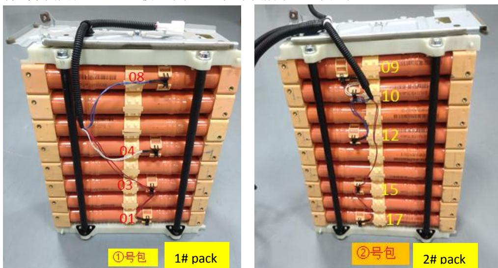
6. Tighten the fixing screws on both sides of the bottom of the module of 1#pack and 2#pack. (Note: torque of screws is 5 ~ 6N•m), as shown below. (将1号包和2号包模组底部两侧固定螺丝进行安装固定，注：螺丝扭力5~6N·m)，如下如图所示。
