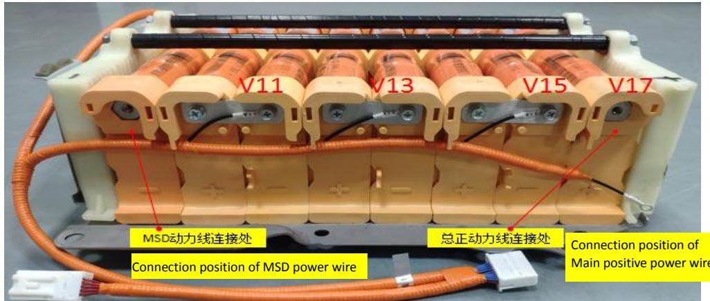
8. Install voltage collection wiring harness and copper busbar on the other side. Note: torque of bronze screw is 5 ~ 6N•m. (安装另一侧电压采集线束及连接铜排, 注: 铜排螺丝拧紧扭力 5~6N • m)。
