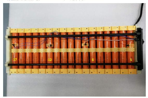
4.3 Tighten the screws at the bottom of module (Note: The torque of screw is 5~6N • M).将模组底部螺丝进行拧紧固定(注:螺丝扭力5~6N • m)。
