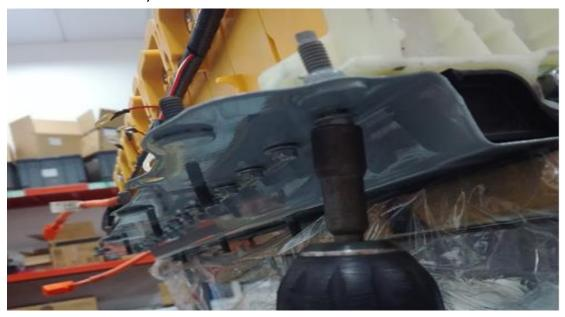
4. 4 Tighten the splint screws at the bottom of module to fix the position. (将定位夹板螺丝进行拧紧固定)。
