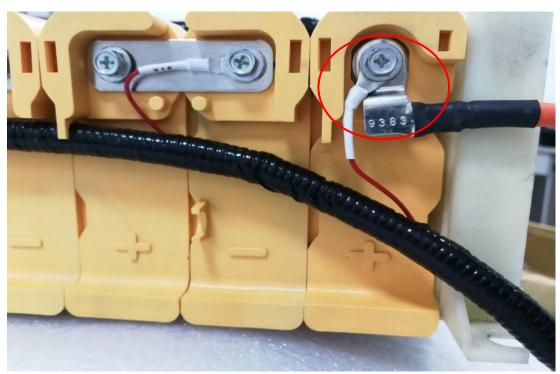
6.3 Install cathode pole connector wire and voltage collection wiring harness #V1. (安装负连接线及电压采集线束 V1)。
