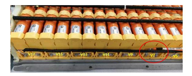
6.2 Install the original voltage collection wire #V18 of the anode pole connector wire. ( 安装原版正连接线电压采集线束 V18)。
