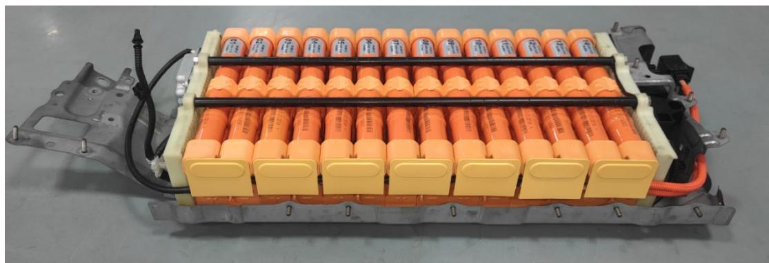
15. Install the plugs of the voltage collection wiring harness and temperature sensors according to the original positions. (按原位置安装电压采集接线插头和温度传感器插头)。
