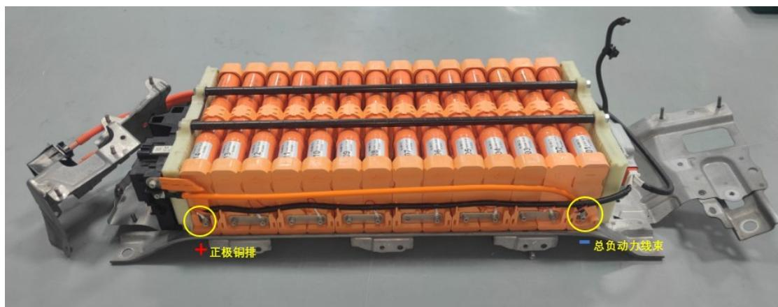
12. Install the main positive and main negative insulation caps at the relay box connection for insulation protection. (安装继电器盒连接处总正、总负绝缘帽，进行绝缘防护)。
