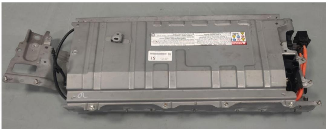
17. Put the battery pack back into the vehicle and connect the main wires of the positive and negative poles in the correct positions. (the correct position are marked with red circle in the follow figure). (完成组装的电池组件，然后放回车辆，正确将正负极接头对插、采集线束接头对插)。
