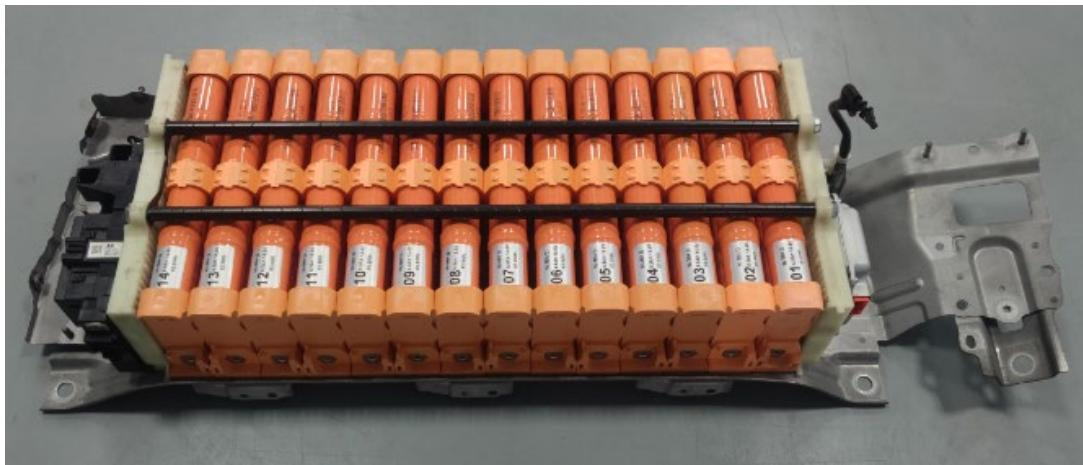
8. Tighten the fixing screws on both sides of the bottom of the modules.
