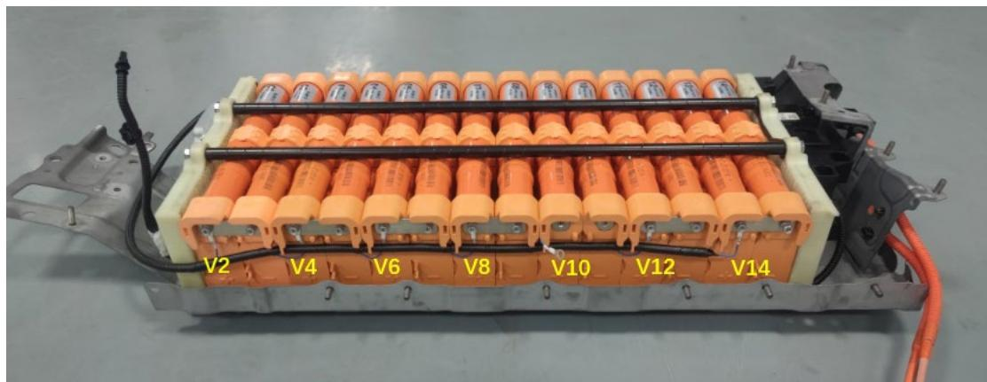
11. Install the positive busbar and the main negative power harness. (安装正极铜排、总负动力线束)。
