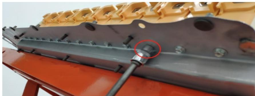
9. Install the voltage collection wiring harness and connector busbars,
