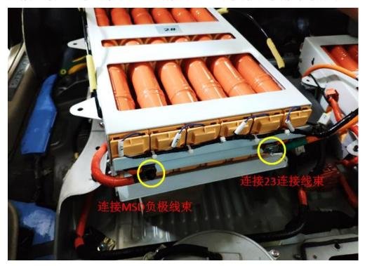
7. Fix the 1#, 2#, and 3# battery box, connect and fix the positive and negative connector wire with main positive connector wire and main negative connector wire of original vehicle respectively, and fix the original car and the main negative cable, then connect the main positive and main negative connector wire's plug fittings of original vehicle to the power distribution box in order of original vehicle. (将 1#、2#、3#箱体进行固定,将正极连接线、负极连接线分别与原车总正、总负连接线连接和固定,原车总正、总负连接线插件按原车顺序连接至配电盒)。
