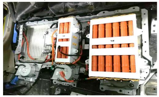
5.1 When installing the 1# battery box: firstly raise the bottom of the battery box with wood, connect the wiring harness terminal of original car's MSD positive terminal to the positive of the 1# battery box, tighten and fix it, protect it with an insulating cap, and install it into the sheet metal case. (安装 1#电池箱时: 电池箱底部用绝缘部件垫高,原车 MSD 正极线束端子连接至 1#电池箱正极位置,拧紧和固定,绝缘帽和绝缘胶带防护,安装至钣金箱体内)。警示: 电池箱总电压超过 115.2V,安装前和安装过程中,须保证: 1#电池箱负极连接线束端绝缘防护完整,否则会出现短路甚至危及人身安全现象。
