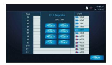
Connect the battery to the device correctly and measure the voltage of each string of batteries at the battery end using a high-precision multimeter. Compared with the voltage displayed on the screen, calibration can be performed when the error is greater than  $\pm 1$ mV. Calibration is insignificant when the error of collected voltage is less than
